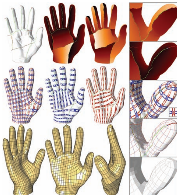
Figure 1: Scanned Hand. From a triangulated surface and a set of line singularities assembled into a singularity graph, our technique solves a linear, modified Laplace equation to get two potentials (top); The pair of 1-forms associated to the potential differentials is specified as either regular, reverse or switch across singularity lines (center). An isocontouring of these potentials results in a pure-quad mesh with non-integer index singularities capturing the geometry (see close-up, right), and no T-junction (bottom).
