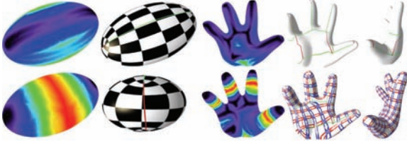
Figure 8: Automatic Generation of Singularity Graph. Left: generation on the ellipsoid. The color map depicts the cumulative distance to the umbilics taking into account the alignment with \kappa_{\min} and \kappa_{\max} . Right: a similar process demonstrated on a cartoon hand.
