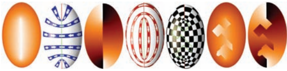
Figure 5: Line Singularity. From left to right: Piecewise-continuous harmonic potentials u and v (color-shaded); Red and blue arrows depict the direction of the potential gradients; a checkerboard is mapped onto the ellipsoid using (u, v) as texture coordinates; when the singularity line is wiggly, the two potential functions change, but their isolines remain exactly identical to the previous case.
