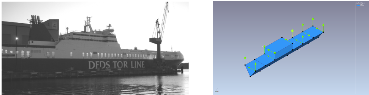
Figure 15: The ship at the Flensburg shipyard (left). The geometry of the ship with 16 acceleration channels in ARTEMIS MODAL PRO 6.0 (right).
