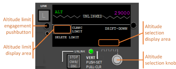
Fig. 3. Panel for altitude management of the ACI device used in this paper.
