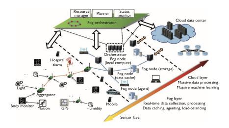
Figure 1: Generic Fog computing architecture [152].
