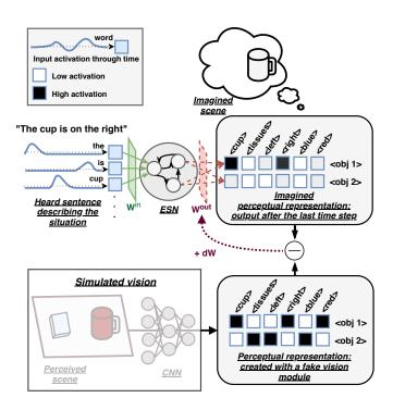
Fig. 2. ResPars adaptation to cross-situational learning. The network is fed a sentence describing a scene it perceives. The difference between the network output and the vision module output is used to update slightly the network weights. By repeating this step on various situations, only the pertinent modifications should be kept, and the network would extract the semantic of the sentences.
