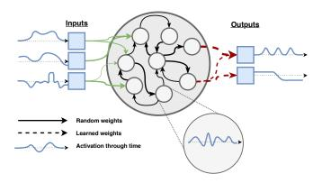
Fig. 1. Reservoir Computing. Echo State Networks are an instance of the Reservoir Computing paradigm using units with continuous states (as opposed to spiking activity). Coherent outputs are generated from the chaotic internal activity.
