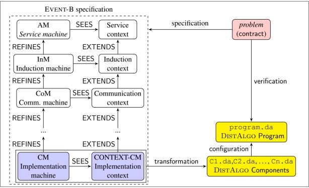
Figure 1: The global methodology for correct-by-construction distributed algorithms.
