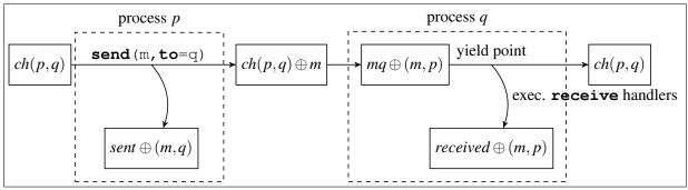
**Figure 2:** Communications in DISTALGO: the communication channels *ch*, as well as the message queues *mq* cannot be accessed explicitly in DISTALGO; only the sent and received messages can be accessed using the **sent** and **received** primitives.
