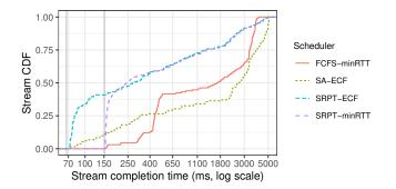
Fig. 9. Simulation of a wikipedia page load by replaying a trace (ID 200413\_FH\_478b18e178c0fbf2ec9312686630e510, run 3, connection 2). Path 0: 1050 Kbit/s, 67 ms. Path 1: 750 Kbit/s, 151 ms. Path latency is indicated with the vertical bars. SRPT-ECF exhibits low completion times, thanks to its combination of ECF (left part of the CDF) and SRPT (tail of the CDF).
