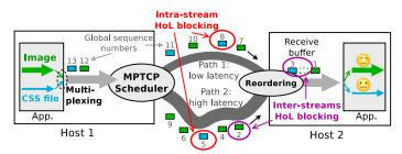
Multipath TCP basic principle, here with data that has been multiplexed by the application. Head-of-Line Fig. 1. blocking can happen both within a stream (packet 8 will arrive before packet 5 for the CSS file) and between streams (packet 3 from the CSS file is waiting for packet 2 from the image).
