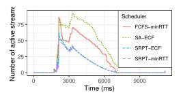
Fig. 10. Scheduler occupation over time during the trace replay. Streams are created in three visible bursts. The schedulers have different strategies for handling the backlog of active streams.
