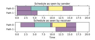
Fig. 8. Optimal schedule obtained by an offline algorithm that minimizes the average completion time. Stream 0 can anticipate the arrivals of Streams 1 and 2, so it uses Path 1 for a longer time to ensure both paths finish at the same time.
