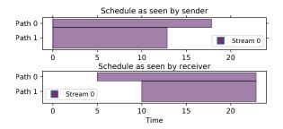
Fig. 3. Example of an optimal schedule computed with ECF for a single stream, as seen from the sender (top) and the receiver (bottom). Notice how data on the two paths completes simultaneously on the receiver side. Path 0 has rate 200 KB/s and latency 5 ms, while path 1 has rate 500 KB/s and latency 10 ms. The stream has a size of 10 KB.
