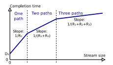
Fig. 4. Completion time as a function of stream size using ECF. Here,  $D_1$  is the delay of the lowest-delay path, while  $R_i$  is the rate (in bit/s) of path *i* where paths are ordered by increasing delay.
