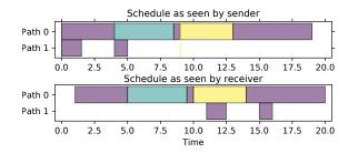
Fig. 7. Example of SRPT-ECF running online. Stream 0 is initially alone and uses ECF as in Fig. 3. When Stream 1 arrives (t = 4), Stream 0 gets preempted immediately: as a result, it starts using Path 1 again so that data on both paths finishes simultaneously, accounting for Stream 1. When Stream 2 arrives (t = 9), Stream 0 is preempted again but this time it is too late to use Path 1, so it just waits for Stream 2 to finish.
