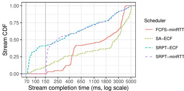
Fig. 9. Simulation of a wikipedia page load by replaying a trace (ID 200413\_FH\_478b18e178c0fbf2ec9312686630e510, run 3, connection 2). Path 0: 1050 Kbit/s, 67 ms. Path 1: 750 Kbit/s, 151 ms. Path latency is indicated with the vertical bars. SRPT-ECF exhibits low completion times, thanks to its combination of ECF (left part of the CDF) and SRPT (tail of the CDF).
