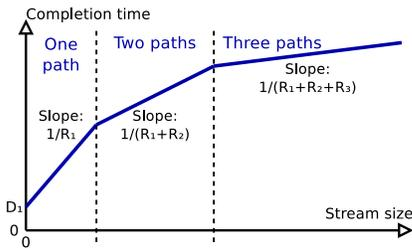
Fig. 4. Completion time as a function of stream size using ECF. Here,  $D_1$  is the delay of the lowest-delay path, while  $R_i$  is the rate (in bit/s) of path  $i$  where paths are ordered by increasing delay.
