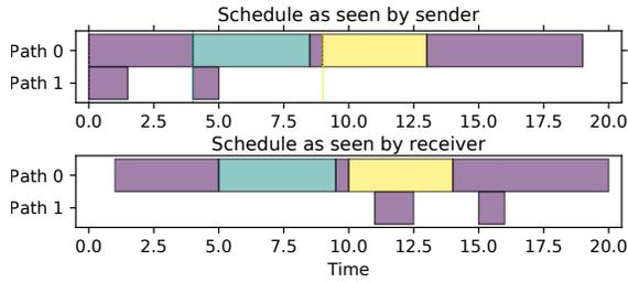
Fig. 7. Example of SRPT-ECF running online. Stream 0 is initially alone and uses ECF as in Fig. 3. When Stream 1 arrives ( $t = 4$ ), Stream 0 gets preempted immediately: as a result, it starts using Path 1 again so that data on both paths finishes simultaneously, accounting for Stream 1. When Stream 2 arrives ( $t = 9$ ), Stream 0 is preempted again but this time it is too late to use Path 1, so it just waits for Stream 2 to finish.
