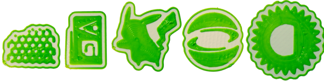
Fig. 19. Photographs of prints obtained on the Ultimaker S5. Because \mathcal{S}^0 is 2\gamma -fat rather than \gamma -fat, a large part of the hexagonal grid is missing; See Figure 15. The second print from the left is 2/3 the scale of the one on Figure 18. This renders the hook \gamma less than 2\gamma -fat in the stem, so that a small part of it has been removed.
