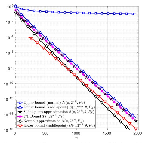
Figure 7: Normal and saddlepoint approximations of the function T in (49) as functions of the blocklength n for the case of a BSC with cross-over probability  $\delta = 0.11$  at information rate R = 0.32 bits per channel use. The channel input distribution  $P_X$  is chosen to be the uniform distribution and  $\theta$  chosen to be the unique solution in t to the equality in (71).
