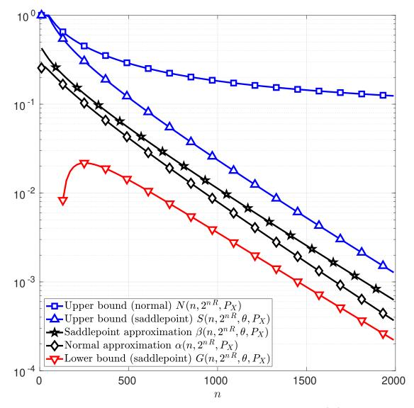
Figure 8: Normal and saddlepoint approximations of the function T in (49) as functions of the blocklength n for the case of a real-valued AWGN channel with discrete channel inputs,  $\mathcal{X} = \{-1, 1\}$ , and SNR = 1 at information rate R = 0.425 bits per channel use. The channel input distribution  $P_X$  is chosen to be the uniform distribution and  $\theta$  chosen to be the unique solution in t to the equality in (71).
