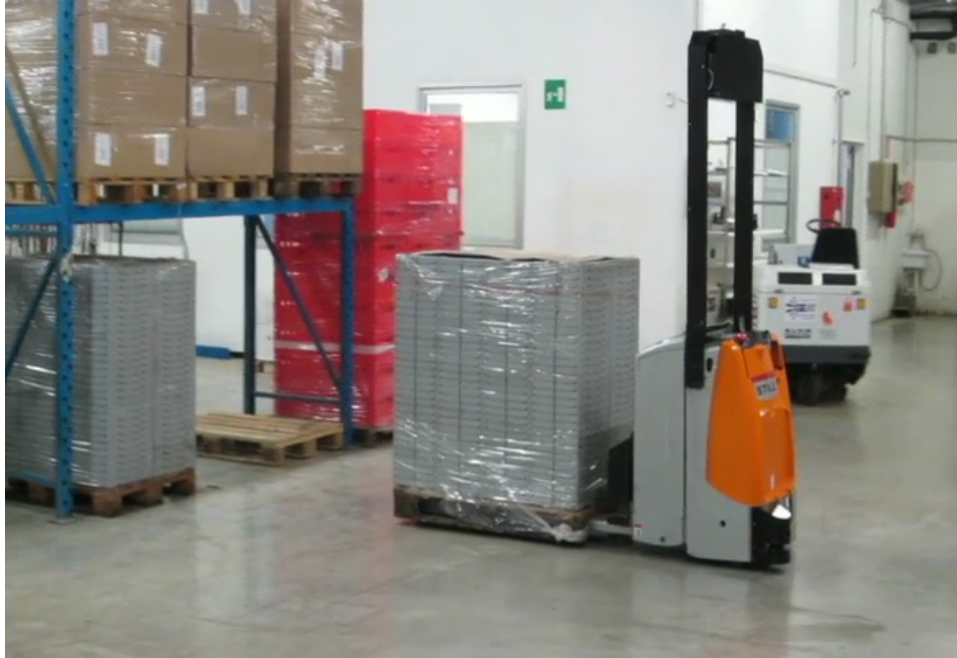
Figure 1.1: The autonomous Trans-pallet for picking up and place pallets inside warehouses
