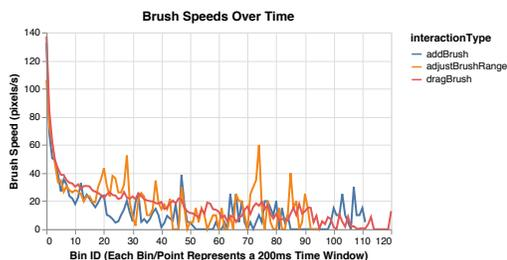
**Figure 3: Average brush speed (in pixels/s) is calculated using windowed aggregation, where each window (or bin) represents a non-overlapping duration of 200 ms. Each bin (i.e., 200ms window) is a single point in the line chart. Insignificant bins in the long tail are hidden to save space (i.e., bin IDs greater than 120, or after a total duration of 24 seconds).**
