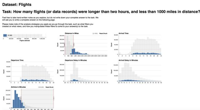
**Figure 1: An example crossfilter application from our user study, visualizing the Flights dataset, composed of six numerical attributes. Each attribute is visualized as a histogram that can be filtered using a range-slider. When the user interacts with a range slider, the entire dataset is filtered, the bins in each histogram are recomputed, and the visualizations are updated.**
