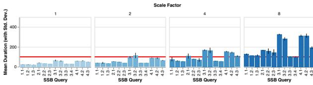
**Figure 7: Mean query duration and standard deviation (in milliseconds) for the 13 queries in the SSB. The mean is calculated across five runs executed for MonetDB. MonetDB performs well (i.e., within our 100ms threshold, drawn in red) up to scale factor four.**
