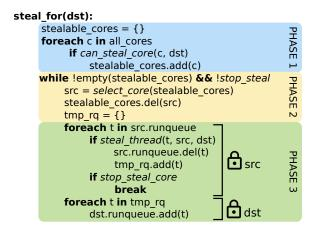
Figure 2. Structure of load balancing
