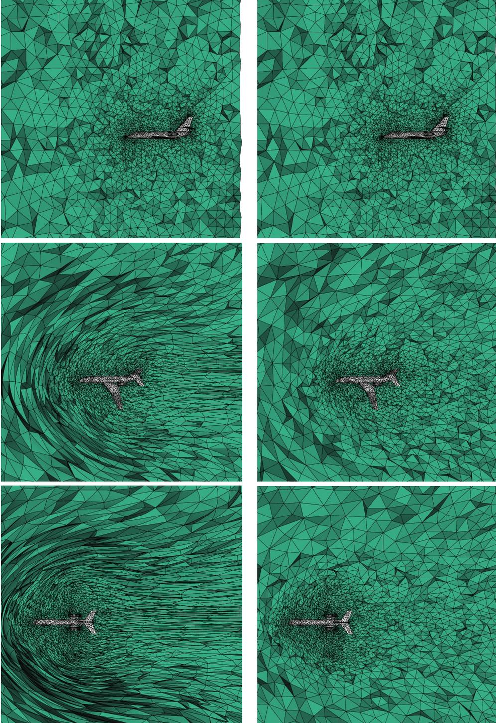
Figure 20: Case of the translating-rotating falcon aircraft inside a  $P^2$  mesh. From top to bottom, zoom in the vicinity of the falcon jet after 0, 25 and 50 iterations of moving-mesh process. Left, without mesh optimization operators. Right, with  $P^2$  mesh optimization operators.
