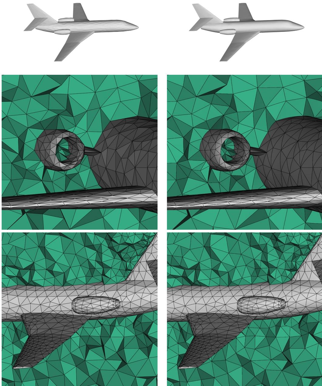
Figure 15: Falcon business jet meshes. From top to bottom, surface and volume meshes. From left to right,  $P^1$  and  $P^2$  meshes.  $P^2$  meshes are generated with Algorithm 1 using a cubic reconstruction.
