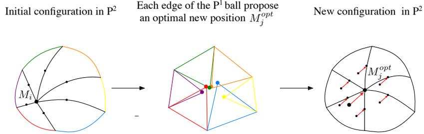
Figure 10:  $P^2$  Laplacian smoothing in two dimensions. Each element of the  $P^1$  ball of considered vertex  $M_i$  suggests an optimal position  $M_j^{opt}$ . The resulting new optimal position  $M_j^{opt}$  is computed as a weighted average of all these proposed locations. The new position of the nodes of the internal edges of the  $P^2$  ball is then deduced by proportionality.
