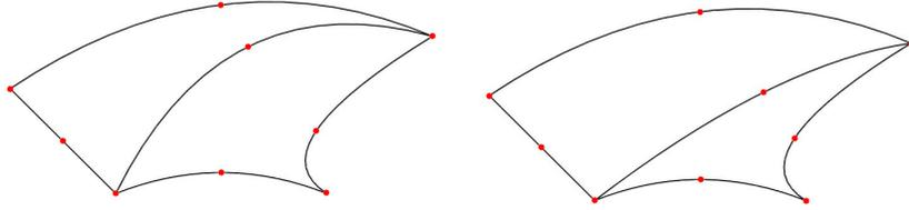
Figure 11:  $P^2$  node smoothing in two dimensions. The optimal position of the node of the central edge is computed solving an optimization problem. Left, the initial configuration, right, the optimized configuration. In the shown case, we have the following initial qualities  $Q_{P^2}^{ini} = 11.34$  and  $4.69$  (left) and the following final qualities  $Q_{P^2}^{end} = 8.36$  and  $2.65$  (right).
