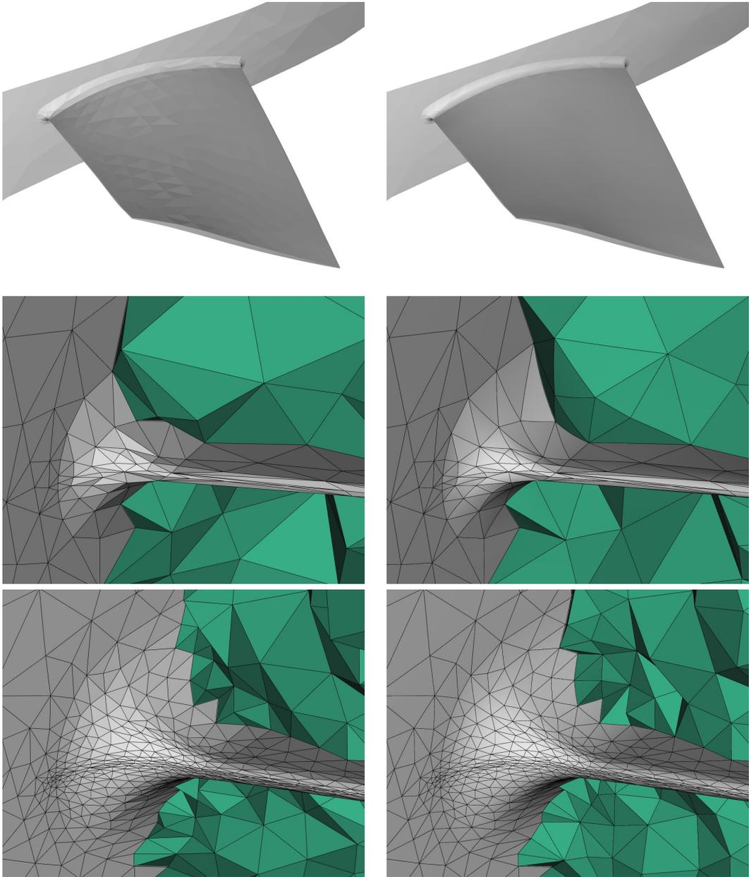
Figure 12: NASA Rotor 37 meshes. From top to bottom, surface, coarse and fine meshes. From left to right,  $P^1$  and  $P^2$  meshes.  $P^2$  meshes are generated with Algorithm 1 using a cubic reconstruction.
