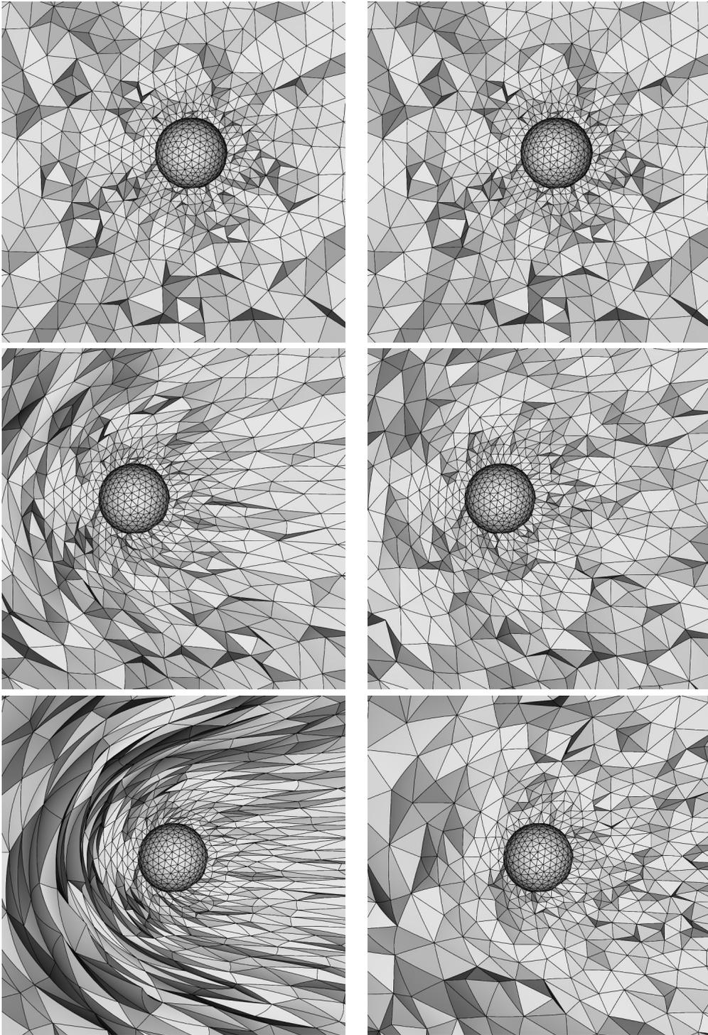
Figure 19: Case of the moving sphere inside a  $P^2$  mesh. From top to bottom, zoom in the vicinity of the sphere at respectively 0 radii, 4 radii and 6.7 radii of displacement. Left, without mesh optimization operators. Right, with  $P^2$  mesh optimization operators.
