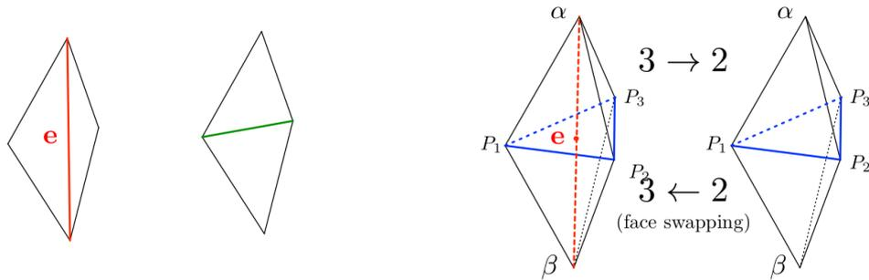
Figure 7: *Left*, the swap operation in 2D. *Right*, edge swap  $3 \rightarrow 2$  and face swap  $2 \rightarrow 3$ . For all these pictures, shells are in *black*, old edges are in *red*, new edges are in *green*.
