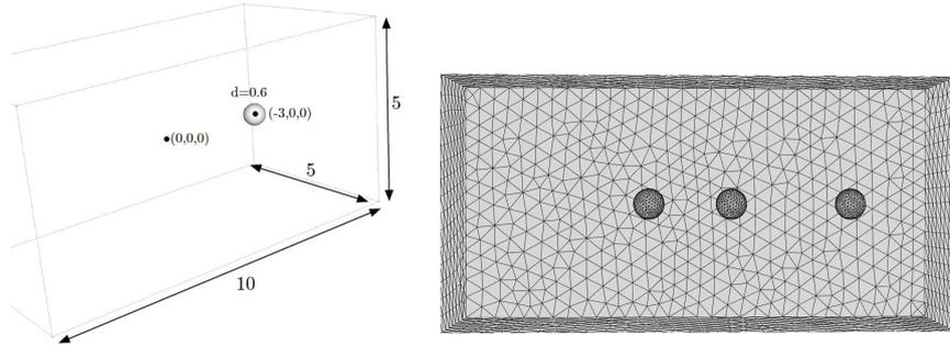
Figure 18: Case of the moving sphere inside a  $P^2$  mesh. Left, description of the geometrical domain. Right, illustration of the three considered positions of the moving sphere where the mesh is analyzed. The sphere is moving from right to left.
