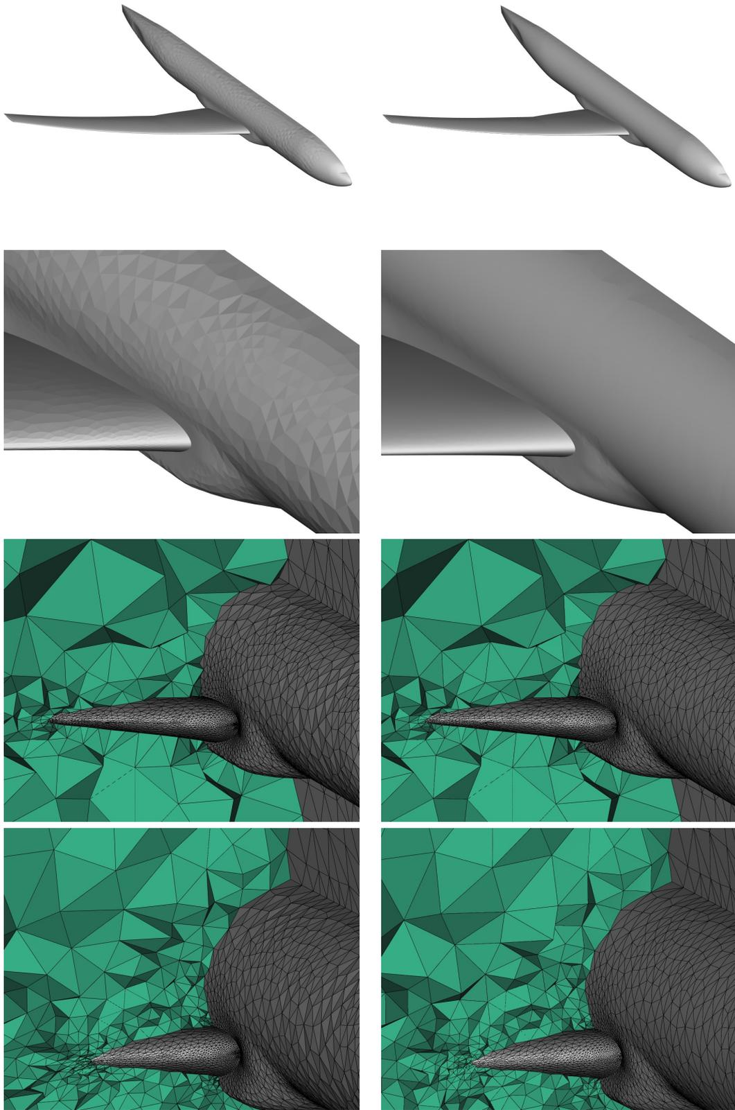
Figure 14: NASA Common Research Model aircraft meshes. From top to bottom, surface, coarse and fine meshes. From left to right,  $P^1$  and  $P^2$  meshes.  $P^2$  meshes are generated with Algorithm 1 using a cubic reconstruction.
