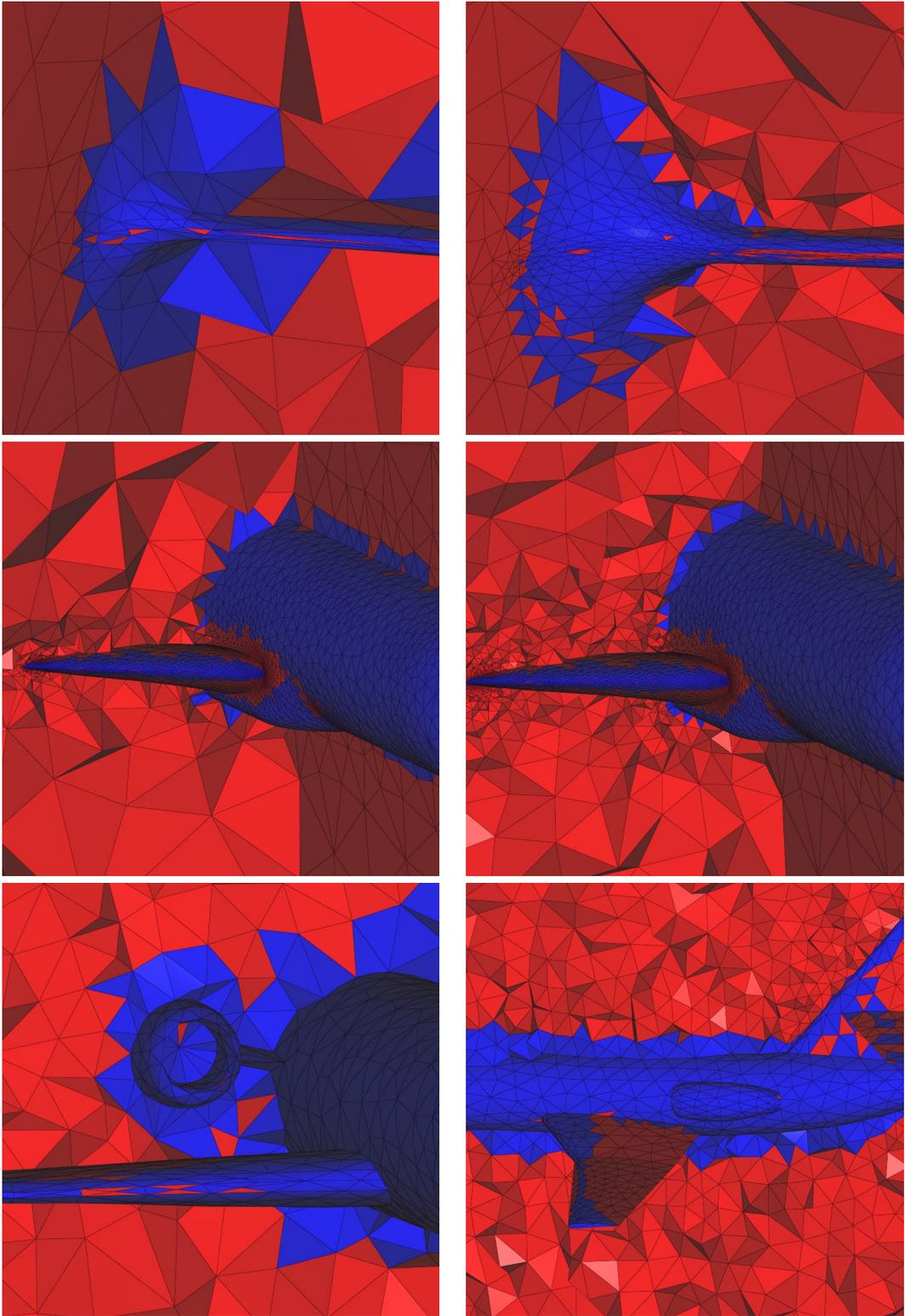
Figure 17: Impact of the mesh curving process for each of the previously studied cases. In red, the volume elements are straight according the straightness criterion of Section 4.1 used with  $\epsilon = 1\%$ . In blue are shown the volume elements that are curved. On each surface triangle is shown the straightness of the volume element generated from it.
