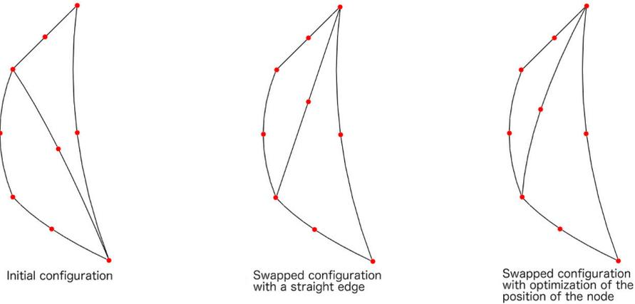
Figure 8: Three steps of  $P^2$  swap in 2D. In the shown case, we have the following qualities  $Q_{P^2}^{ini} = 10.45$  and  $6.04$  (left), then  $Q_{P^2}^{mid} = 5.78$  and  $4.48$  (middle) and finally  $Q_{P^2}^{end} = 4.78$  and  $3.72$  (right).
