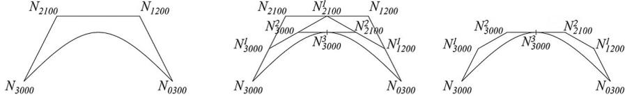
Figure 6: De Casteljau's refinement on two control coefficients of the Jacobian curve on a curved edge of a  $P^2$  tetrahedron. Left, the initial curve with its control coefficients. Middle, construction of the new control coefficients. Right, the initial curve divided in two curves with their control coefficients.
