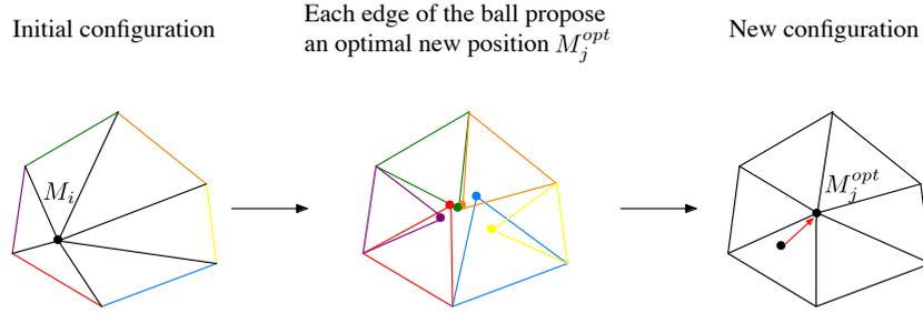
Figure 9: Laplacian smoothing in two dimensions. Each element of the ball of considered vertex  $M_i$  suggests an optimal position  $M_j^{opt}$ . The resulting new optimal position  $M_i^{opt}$  computed as a weighted average of all these proposed locations using Relation (7).
