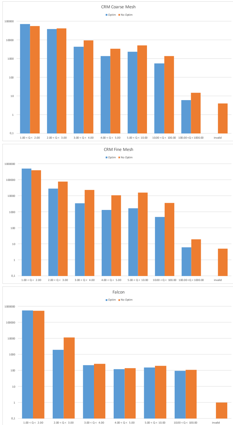
Figure 16: Charts showing the distribution of mesh quality for the cases involving the NASA Common Research Model and the Falcon with or without optimization. The y -axis gives the number of elements. In blue, the charts show the results with optimization. In orange, the charts show the results without optimization.
