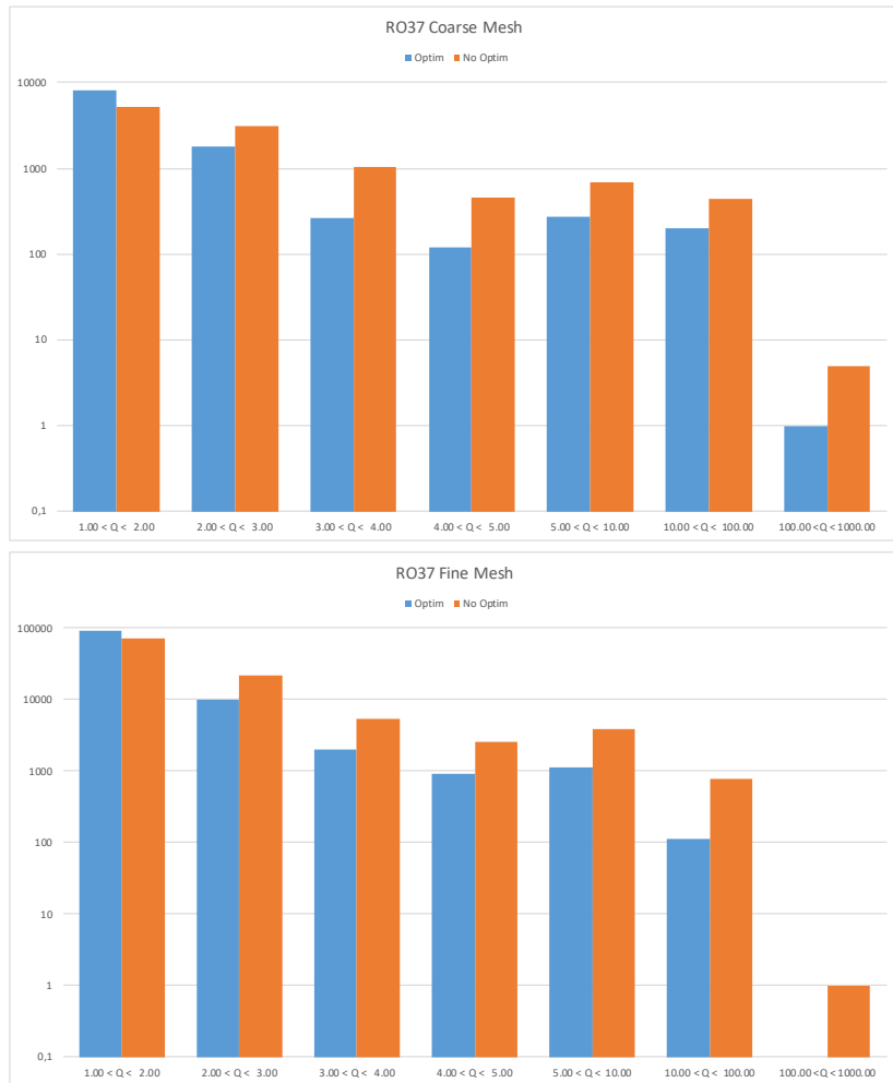
Figure 13: Charts showing the distribution of mesh quality for the two cases with the NASA Rotor 37 with or without optimization. The y -axis gives the number of elements. In blue, the charts show the results with optimization. In orange, the charts show the results without optimization.
