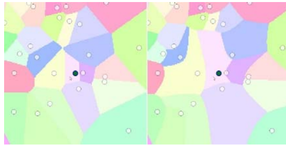
Fig. 3. Different effective areas defined by the unweighted Voronoi diagram ( left ) and the additive weighted Voronoi diagram ( right ).
