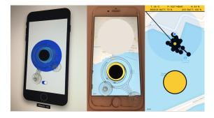
**Fig. 3.** Seamote App - An evolution of a mobile application GUI. From left to right: using a joystick mounted with a tangible analog stick using silicon suction cups. Image to the right: a map depicting the latitude and longitude of the Seamote USV.
