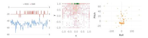
**Fig. 6.** Signal to Noise Ratio (SNR) consistent across different Received Signal Strength Indicator (RSSI) in water environments. **Fig.7.** X and Y map of the commands sent from the mobile application. Color and size denote the usage frequency of those positions (green indicating more). **Fig.8.** USV pitch and roll indicating a tendency to lean backwards, as the primary motion in the tests was a forwards motion.
