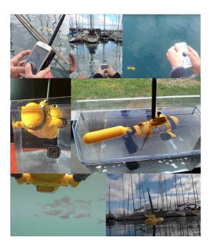
**Fig. 2.** Seamote USV - Deployed in-situ, used for the preliminary tests with participants. Top: Seamote App, used from the marina standpoint. Middle: Seamote USV buoyancy and stability tests. Bottom: Underwater imagery collected by the participants and Seamote USV against other marine vessels found in local marina.
