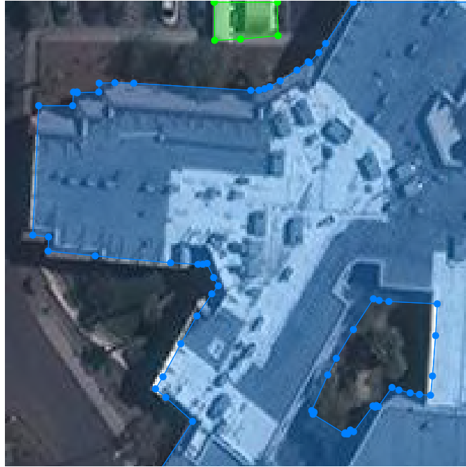
(a) Ours : UResNet101 with frame field learning (full) and frame field polygonization
