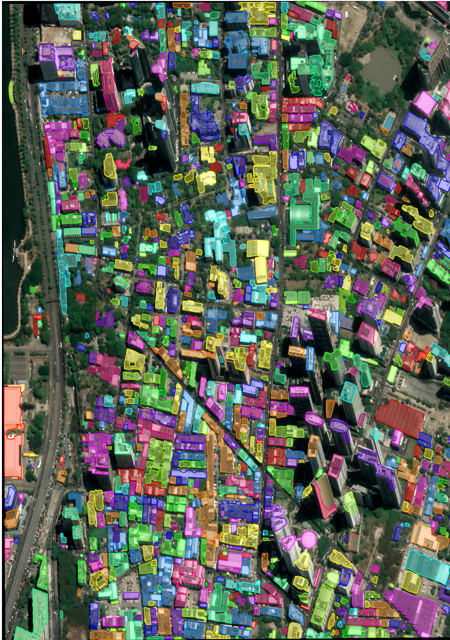
Fig. S8: U-Net16 Baseline (no field): the simple polygonization method with no frame field learning on the “Bangkok” test image from the private dataset with a simplification tolerance of 1 pixel.
