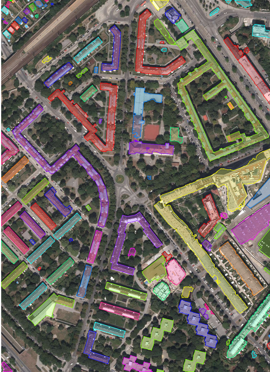
Fig. S4: U-Net16 baseline (no field): the baseline polygonization method with no frame field learning on a crop of the vienna36 test image from the Inria dataset with a simplification tolerance of 1 pixel.
