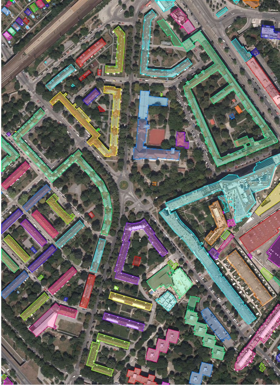
Fig. S3: U-Net16 Ours (full): our full method on a crop of the vienna36 test image from the Inria dataset with a simplification tolerance of 1 pixel.
