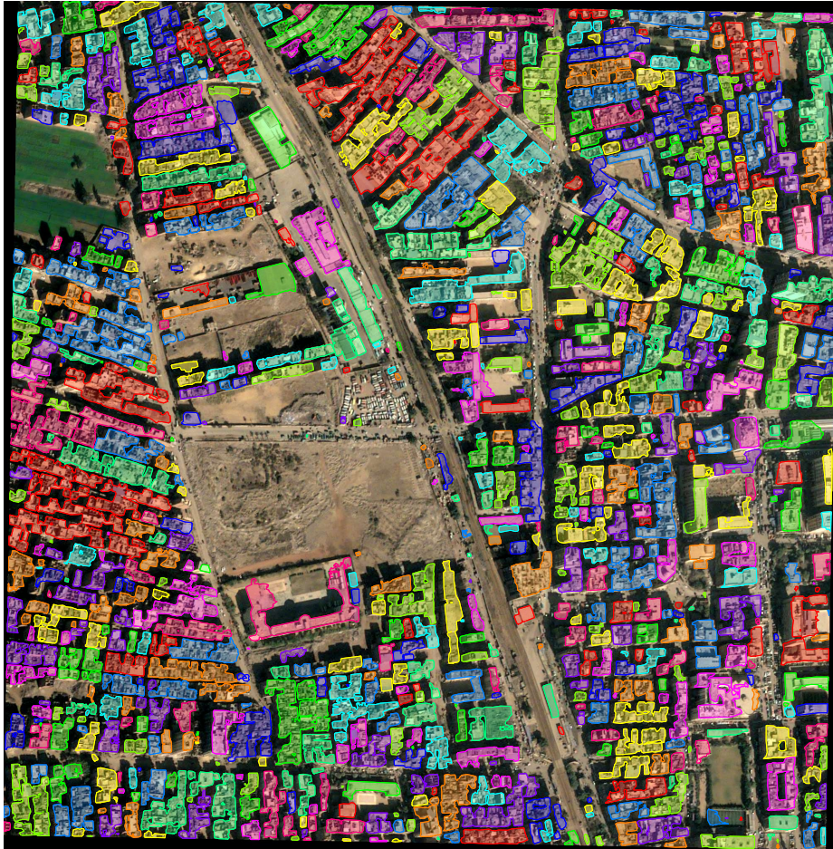
Fig. S6: U-Net16 Baseline (no field): the simple polygonization method with no frame field learning on the “Egypt” test image from the private dataset with a simplification tolerance of 1 pixel.
