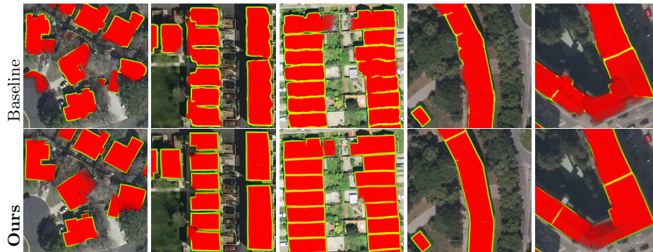
Fig. 7: Predicted classification maps (red: interior, green: boundary) on a few test patches (zoom for details). First row is the baseline U-Net16 with no frame field, second row is our U-Net16 with frame field learning.
