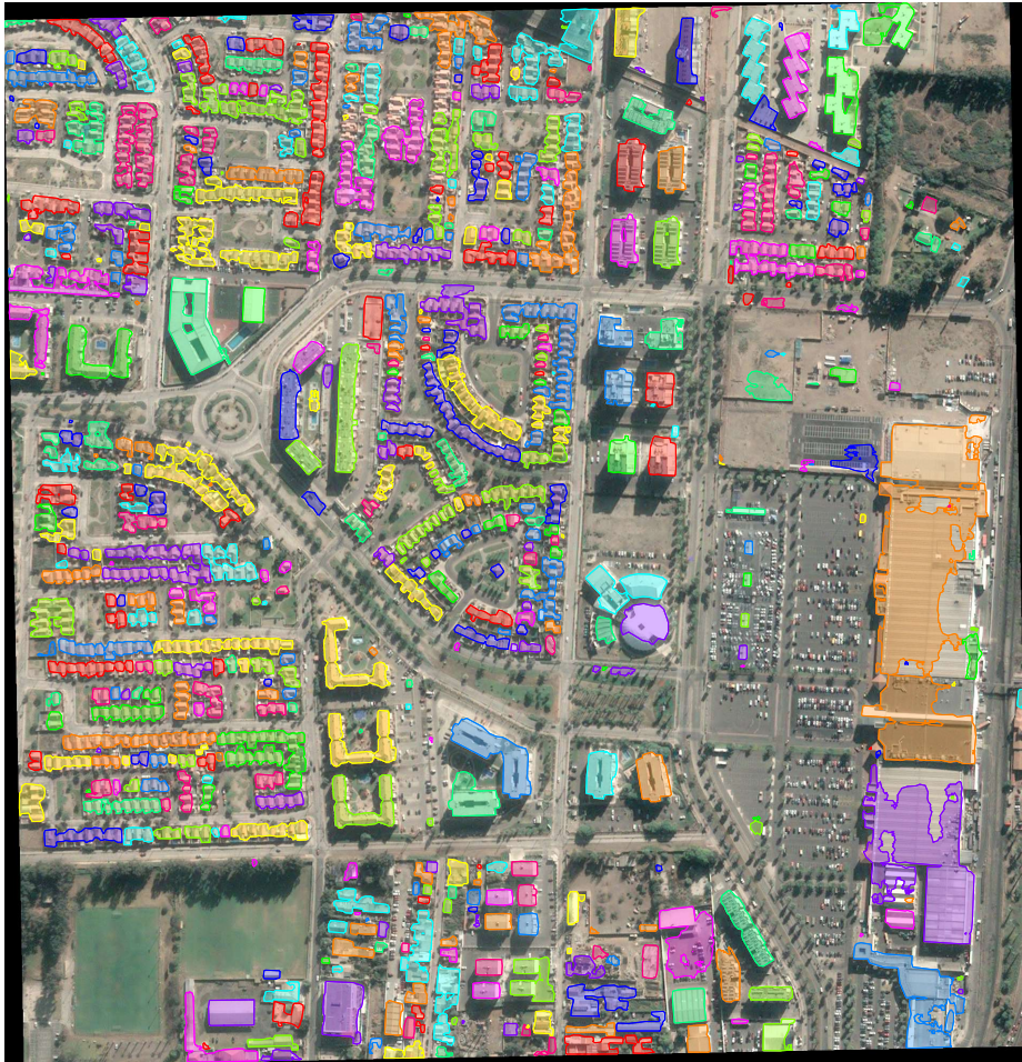
Fig. S10: U-Net16 Baseline (no field): the simple polygonization method with no frame field learning on the “Chile” test image from the private dataset with a simplification tolerance of 1 pixel.
