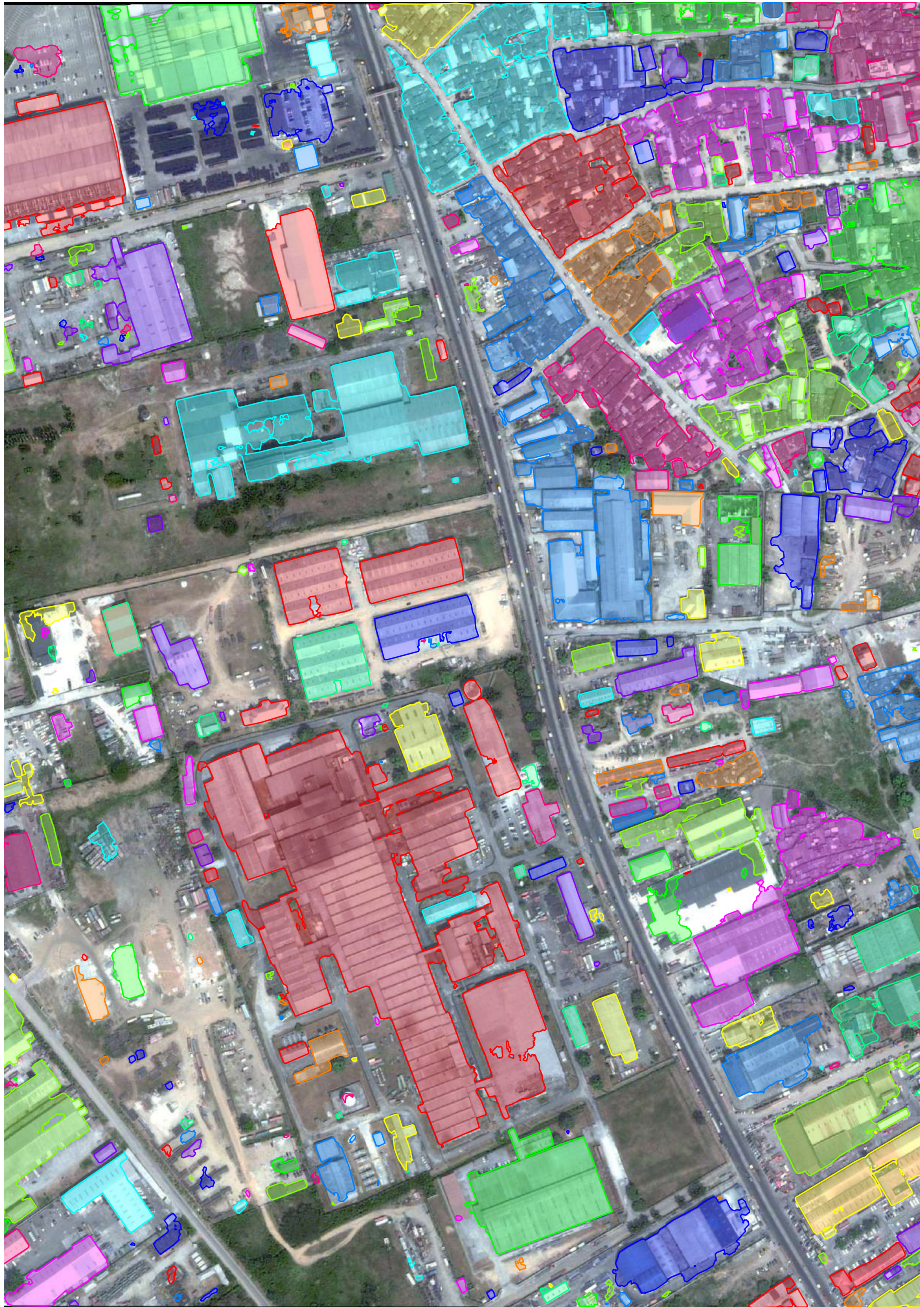
Fig. S12: U-Net16 Baseline (no field): the simple polygonization method with no frame field learning on the “PortHarcourt” test image from the private dataset with a simplification tolerance of 1 pixel.
