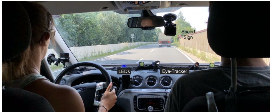
Fig. 1. Setup in the car. The gaze of the front-seat passenger is captured with an eye-tracking system and is visualized for the driver with blue glowing LEDs on an LED-strip mounted at the bottom of the windshield. The front-seat passenger is currently looking at the speed sign ahead on the right side of the street.
