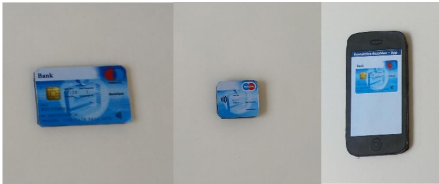
Fig. 4. NFC components a) NFC card b) NFC sticker c) NFC mobile App
