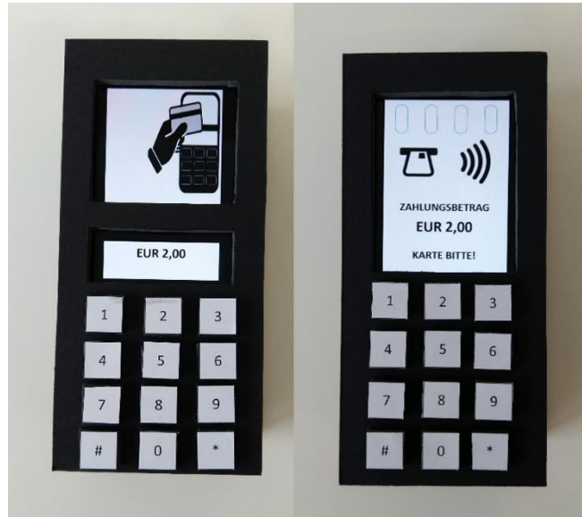
Fig. 3. a) Screen design prototype with a modified screen design. b) Base prototype – replication of the payment terminals used in supermarkets and cafes.
