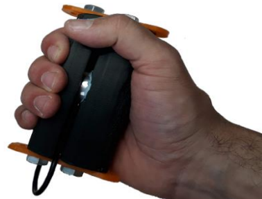
Fig. 4. Hand dynamometer used to measure hand grip strength..
