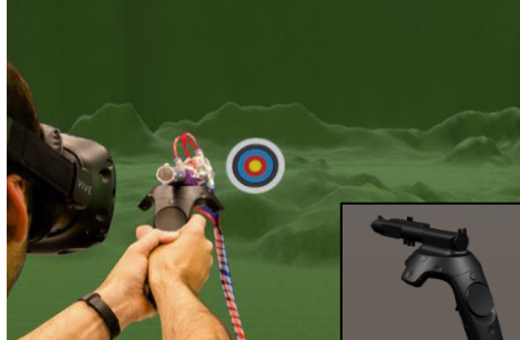
Fig. 1. Force feedback device and the environment used to test the effects of recoil on shooting performance. Right button corner, in-game visual representation of the controller, replicating the shape of the physical prototype.
