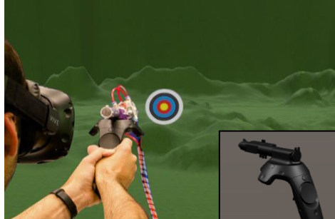
Fig. 1. Force feedback device and the environment used to test the effects of recoil on shooting performance. Right bottom corner, in-game visual representation of the controller, replicating the shape of the physical prototype.
