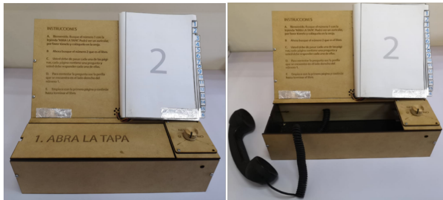
Fig. 1. Aestimo : tangible interface kit (33.9 cm, 26 cm, 23.8 cm).
