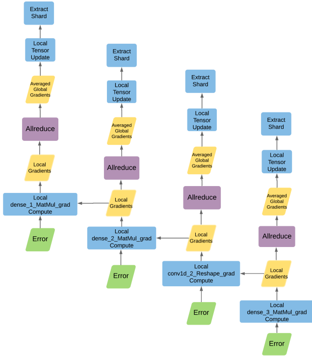
Fig. 3: Example: fine-grain sharding during back-propagation, including the pipeline between the shards.
