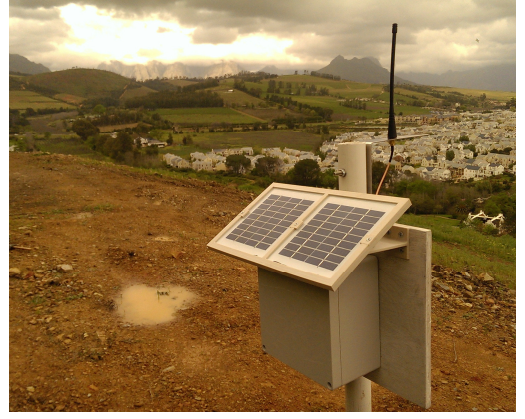
Fig. 8. A photograph showing one of the LoRa field nodes used in our outdoor experimental evaluation.
