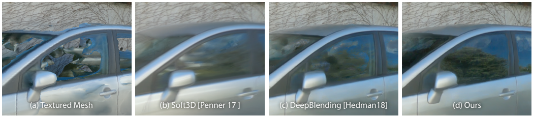
Fig. 1. We propose a new solution for rendering captured cars, and in particular their reflective, semi-transparent windows. A textured mesh from multi-view stereo reconstruction (a) is missing the window geometry. Recent free-viewpoint Image-Based Rendering algorithms (b, c) are not designed to handle the rendering of both the reflection of blue sky, green leaves and the transmissive content (car interior). Our method (d) handles this by computing real-time reflection flows on an ellipsoid approximation of the curved window surface, based on our estimate of a smooth hull of the car that exploit semantic labels in the input images. The effect of reflection rendering is best seen in the supplemental videos.
