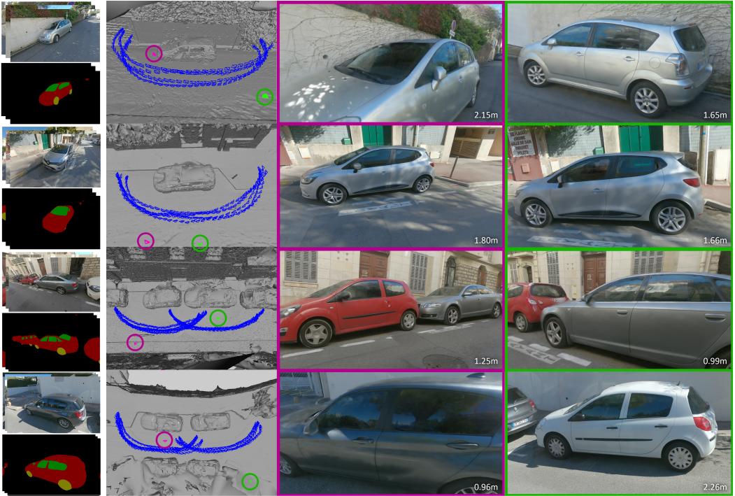
Fig. 10. Our scenes, top to bottom: Vine , Carpenter , Narrow-Street and Corner-Street . Left to right: input images and semantic masks, scene geometry with the input viewpoints (in blue) and output viewpoints (pink and green), two renderings of each scene using our method. Note the distance from each novel view to the closest input viewpoint (displayed in overlay).
