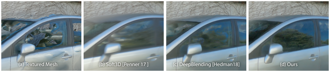
Fig. 1. We propose a new solution for rendering captured cars, and in particular their reflective, semi-transparent windows. A textured mesh from multi-view stereo reconstruction (a) is missing the window geometry. Recent free-viewpoint Image-Based Rendering algorithms (b, c) are not designed to handle the rendering of both the reflection of blue sky, green leaves and the transmissive content (car interior). Our method (d) handles this by computing real-time reflection flows on an ellipsoid approximation of the curved window surface, based on our estimate of a smooth hull of the car that exploit semantic labels in the input images. The effect of reflection rendering is best seen in the supplemental videos.
