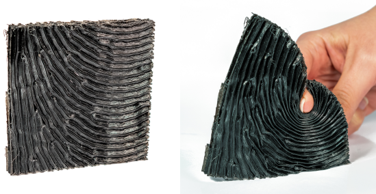
Fig. 22. A structured plate. The orientations produce a strong collapsing/gripping effect when pressing on a specific location.
