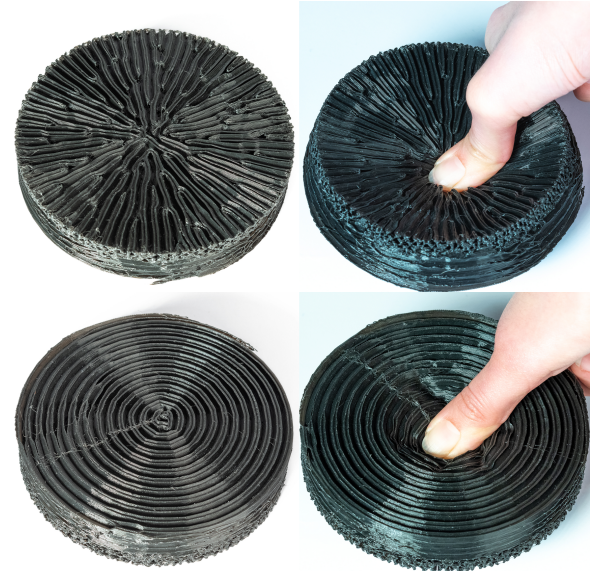
Fig. 24. Top : Thick disc with radial fiber pattern. Pressing in the center lifts the sides up. Bottom : With a circular direction field, the central pressure is absorbed and has no effect on the sides.
