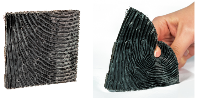
Fig. 27. A structured plate. The orientations produce a strong collapsing effect when pressing on a specific location.
