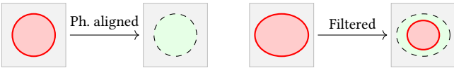
Fig. 15. Effect of removing a singularity vs. changing its shape. Given our metric \mathcal{S} , removing a singularity through phase alignment has a large impact on the cumulative count of pixels above the threshold (left, green). Filtering a singularity which cannot be removed changes its shape and reduces its area slightly, although with a much smaller impact on the cumulative count (right, green). This however greatly reduces the profile distortion that happens in the result (Figure 11).
