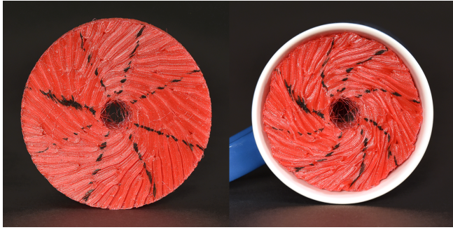
Fig. 28. A wheel design with a spiraling direction field. Left: The structure at rest, with black lines drawn on it to better outline the deformation. Right: The wheel under radial compression. Note the spiraling effect occurring due to the deformation being concentrated orthogonally to the spiraling transverse rigidity.
