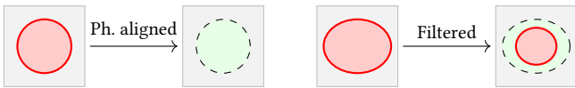
Fig. 15. Effect of removing a singularity vs. changing its shape. Given our metric \mathcal{S} , removing a singularity through phase alignment has a large impact on the cumulative count of pixels above the threshold (left, green). Filtering a singularity which cannot be removed changes its shape and reduces its area slightly, although with a much smaller impact on the cumulative count (right, green). This however greatly reduces the profile distortion that happens in the result (Figure 11).
