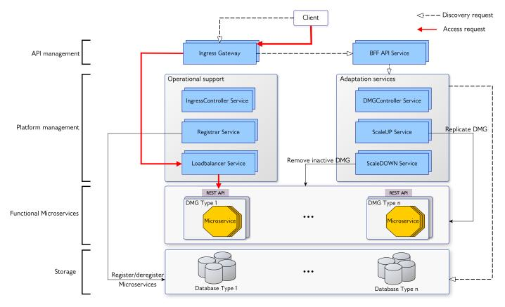
Fig. 3: Overview of the data-driven QoS architecture. It provides operational and adaptation support to control the discovery and access requests initiated by the clients.
