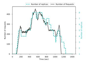
Fig. 5: With a dynamic incoming rate, the system tune the number of replicas according to the load.
