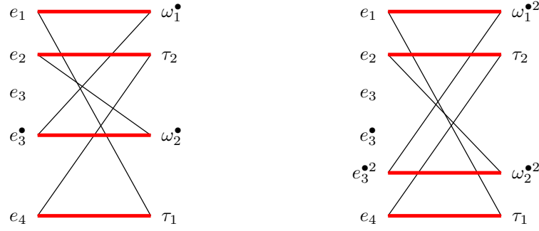
Figure 24: The clutch is an example in which c_f^- = c_f holds. Maximal cardinality matchings for N = 1 (left) and N = 2 (right) are given. Subsequently applying the Dulmage-Mendelsohn decomposition returns \beta_{\mathfrak{D}} = \{e_3\} on the left, and \beta_{\mathfrak{D}} = \{e_3, e_3^{\bullet}\} on the right.
