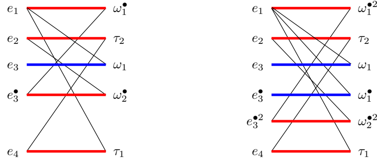
Figure 24: An example with c_f^- < c_f : a variation on the clutch. The previous mode does not involve \omega_1^\bullet , hence \omega_1 remains a dependent variable when entering the new mode. Maximal cardinality matchings for N = 1 (left) and N = 2 (right) are shown. With reference with the example of Figure 23, the added edges correspond to consistency equations and are colored in blue. Subsequently applying the Dulmage-Mendelsohn decomposition returns \beta_\Sigma = \emptyset on both. Actually, the two matchings are complete. As a result, the mode change is fully determined, despite the new mode for the clutch having underdetermined consistency conditions (because the common rotation velocity is free).
