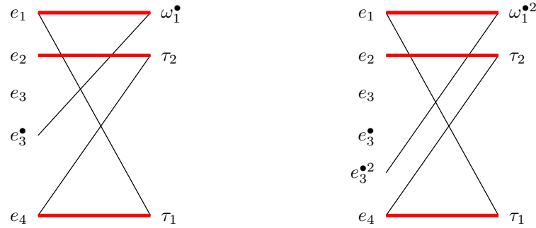
Figure 25: An example with c_f^- > c_f : another variation on the clutch. The previous mode determines \omega_2^{2\bullet} , hence \omega_2^\bullet is no longer a dependent variable when entering the new mode. Maximal cardinality matchings for N = 1 (left) and N = 2 (right) are shown. Subsequently applying the Dulmage-Mendelsohn decomposition on the left-hand graph returns \beta_\Sigma = \mathcal{G}_F , hence Line 6 of Algorithm 10 returns H = \emptyset . No equation of the new mode is satisfied at the first instant and we move to the next instant. The same holds for the right-hand graph.
