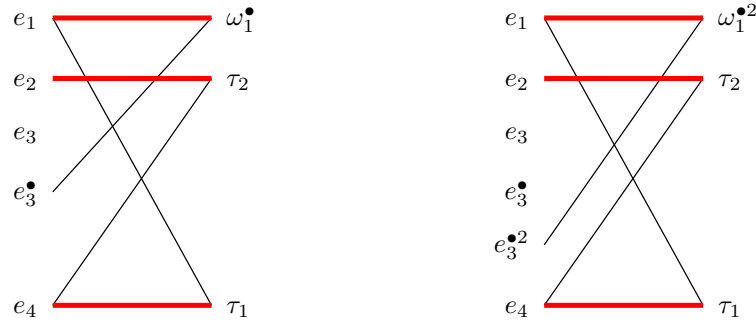
Figure 25: An example with c_f^- > c_f : another variation on the clutch. The previous mode determines \omega_2^{\bullet^2} , hence \omega_2^\bullet is no longer a dependent variable when entering the new mode. Maximal cardinality matchings for N = 1 (left) and N = 2 (right) are shown. Subsequently applying the Dulmage-Mendelsohn decomposition on the left-hand graph returns \beta_\Sigma = \mathcal{G}_F , hence Line 6 of Algorithm 10 returns H = \emptyset . No equation of the new mode is satisfied at the first instant and we move to the next instant. The same holds for the right-hand graph.
