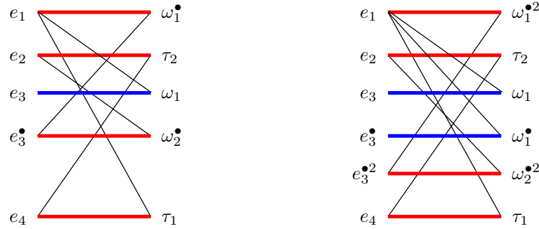
Figure 25: An example with c_f^- < c_f : a variation on the clutch. The previous mode does not involve \omega_1^\bullet , hence \omega_1 remains a dependent variable when entering the new mode. Maximal cardinality matchings for N = 1 (left) and N = 2 (right) are shown. With reference with the example of Figure 24, the added edges correspond to consistency equations and are colored in blue. Subsequently applying the Dulmage-Mendelsohn decomposition returns \beta_\Sigma = \emptyset on both. Actually, the two matchings are complete. As a result, the mode change is fully determined, despite the new mode for the clutch having underdetermined consistency conditions (because the common rotation velocity is free).
