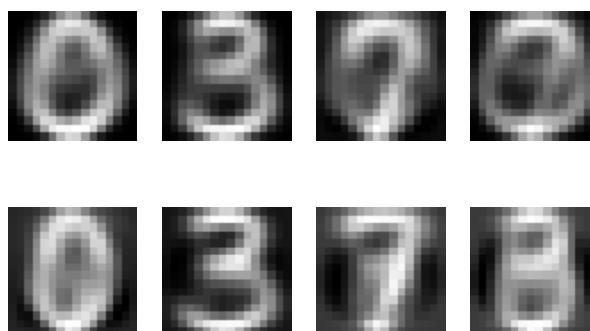
Figure S17. Estimated sources by EM (up) and tmp-EM (down). The "8" and the "7" in particular were much better identified by tmp-EM. Moreover, with tempering the "0" has a more symmetrical shape and the "3" is sharper and less ambiguous.
