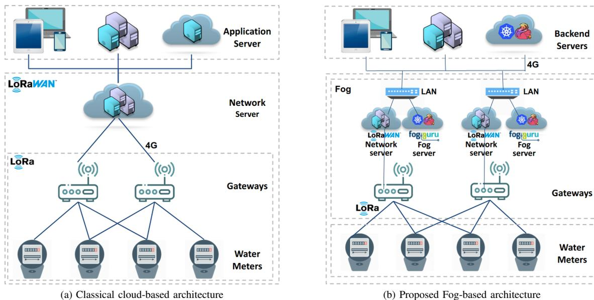
Fig. 1: Two potential system architectures.
