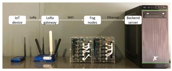
Fig. 2: The experimental testbed.
