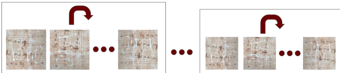
Figure 8: Matching is performed at five scales of the original photograph, each including 90^\circ rotation and horizontal and vertical flipping.
