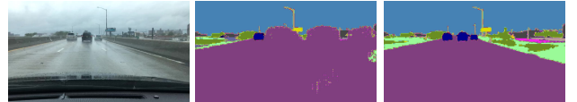
Fig. 6: BDD sample. Left: RGB in rainy; Center: No adaptation; Right: DLV3 MMD rainy adaptation.
