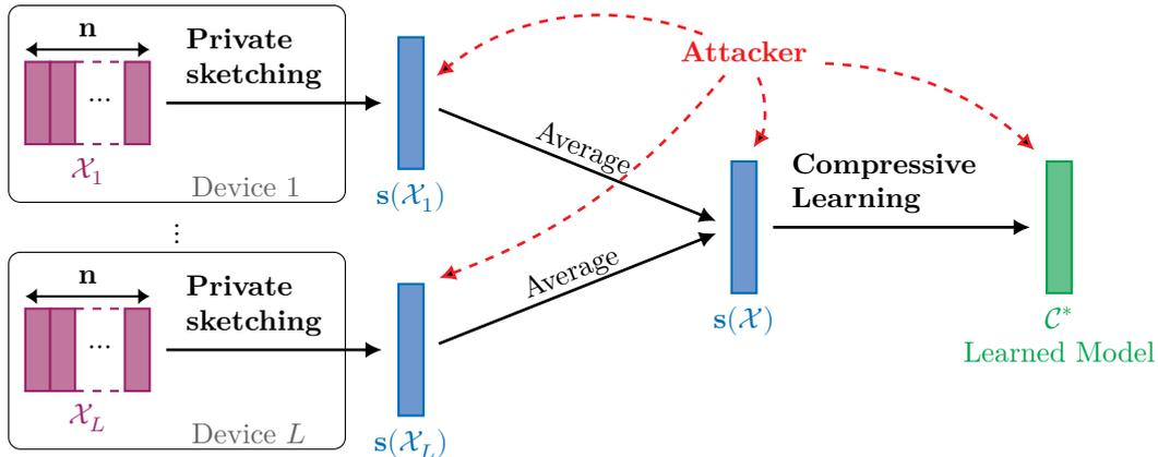
Figure 2: Attack model. The dataset is distributed between  $L$  devices, each computing and releasing publicly a subsampled sketch  $\mathbf{s}(\mathcal{X}_i)$ .
