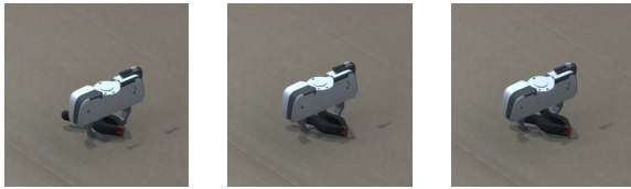
Fig. 4. Example of predefined successful gripper poses used for training the DRL agent in simulator.
