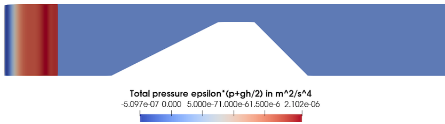
Fig. 5 Variations of the quantity x \mapsto \varepsilon(p + gh/2) with \varepsilon = 10^{-7} \text{ m}^{-2} \cdot \text{s}^2 at time t = 0.01 \text{ s} .
