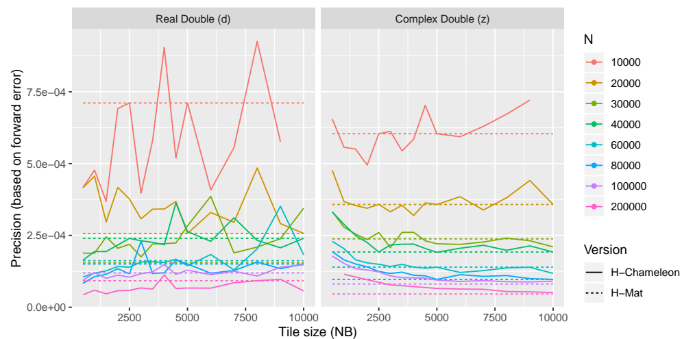
Figure 5: Comparison of the precision of the solver (based on forward error) between H-MAT-OSS original clustering algorithm (dashed line) and \mathcal{H} -CHAMELEON ntils clustering algorithm (full lines) in function of the tile size, for double precision (left) and complex precision (right).
