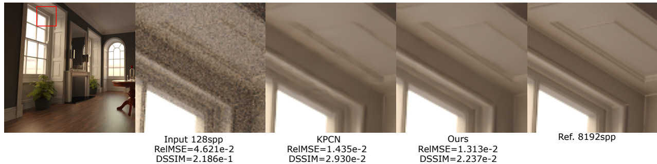
Fig. 1 Comparison between our network and Kernel Predicting Convolutional Network (KPCN) [2]. KPCN and our model use the same dataset for training. Our model preserves details better, due to the novel network structure, a new feature (light transport covariance in path space) and the perceptual loss function. The error metrics (RelMSE and DSSIM) also confirm the higher quality of our method.
