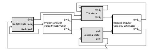
Fig. 4. Supervision of the different phases of the motion and their transitions. If the tilt velocity  $\dot{\psi}$  is beyond a limit  $\dot{\psi}_l$ , the controller transitions directly to the "tilt" state. Below this limit, the choice between the "tilt" state and the "landing" state depends on the impact velocity limit  $\dot{\psi}_{lim}$ .
