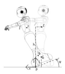
Fig. 3. When the robot tilts, the CoP p lies on the tilting axis. In order to simplify notations, we consider that tilting occurs around two wheels in the direction of the x axis, with an angle  $\psi \ge 0$ .
