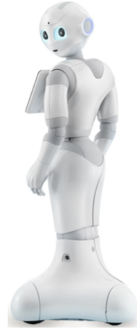
Fig. 1. Pepper is a humanoid robot standing on a holonomic mobile base, equipped with three omnidirectional wheels. It is developed by Aldebaran Robotics for the Japanese Telecommunication Company Soft Bank, to welcome customers in their shops.
